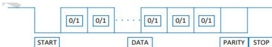
Figure 15 LPUART data transmission format
